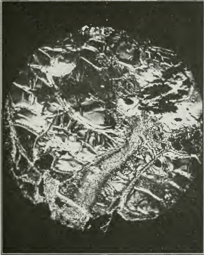
Microphotograph of serpentine close to asbestos vein, Dr. Reed's mine. Magnified 50 diameters. For description see page 46.
